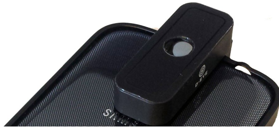
Figure 1. Galaxy S4 equipped with the D-Eye adapter. The D-Eye adapter is magnetically attached to a frame that encompasses the Galaxy S4.
